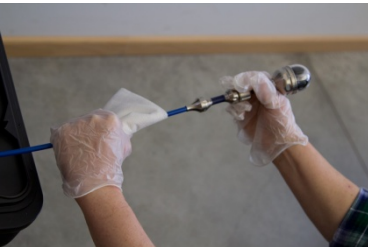
Grasp the rod or cable with a tissue and pull the rod bag into the case
